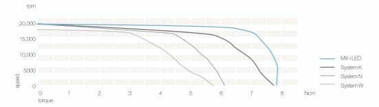
The MX-i LED micromotor is first and foremost a model of stability. It offers great working comfort at both high and low speeds. The high torque of the new MX-i LED makes it one of the most powerful micromotors on the market. Depending on the torque needed, the power is regulated and stabilised by the electronic system. This allows the speed to be maintained with great precision throughout the operation.
